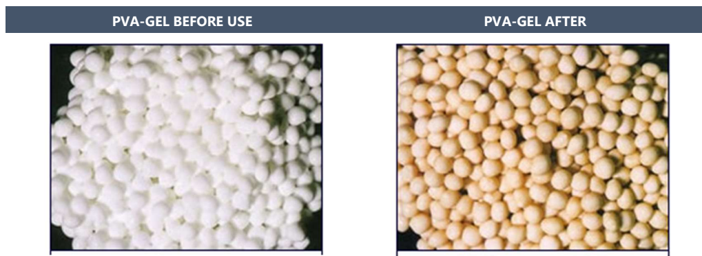
Figure 1: PVA-GEL image before and after one month inside a bioreactor (Kuraray Aqua Co., 2023)
